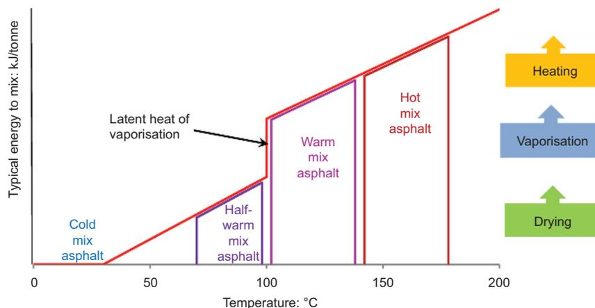
Figure 1. Classification by temperature range
