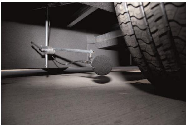
Figure 6. Position of one of the microphones near the reference tyre of the CPX trailer.
