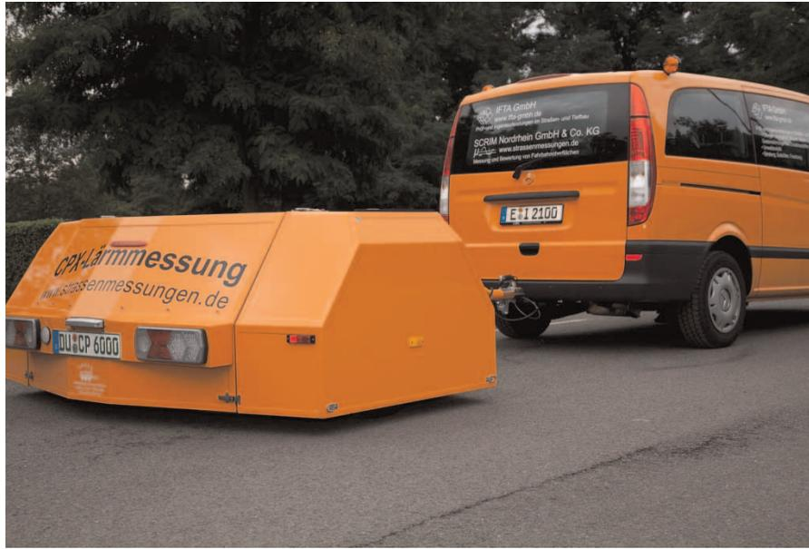
Figure 5. IFTA measuring trailer with towing vehicle used for the CPX measurements.
