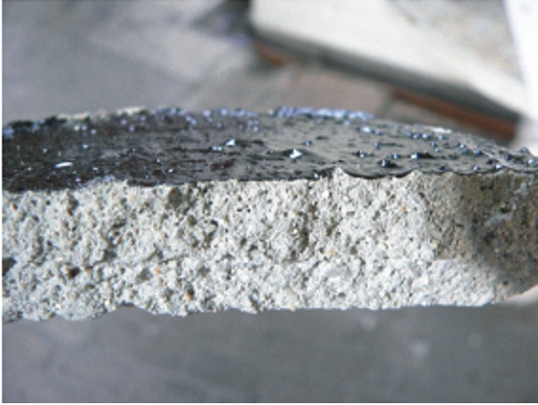
Figure 1: Non-penetrating effect of an 'oil-in-water' bitumen emulsion
