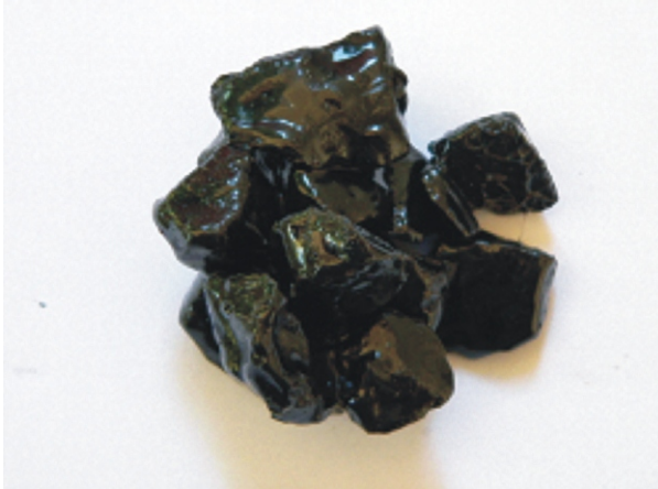
Figure 3: Influence of an adhesion agent on precoated aggregate after the stripping test
