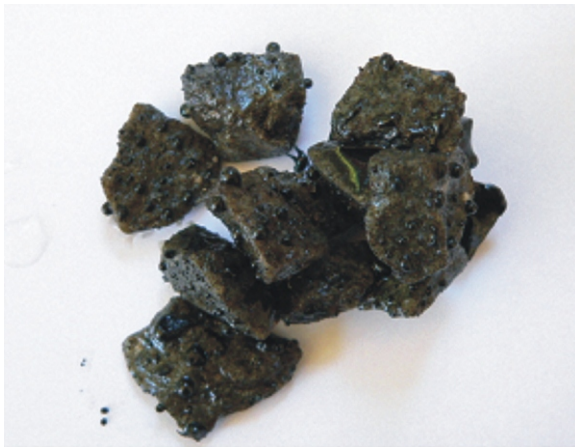
Figure 4: Precoated aggregate without adhesion agent after the stripping test
