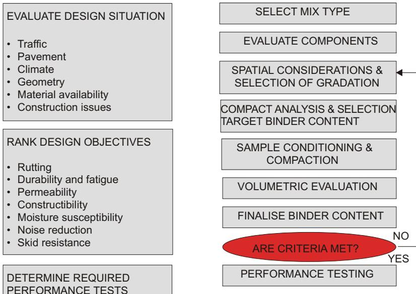
The selection of the mix type can be optimised by considering the design objectives which are influenced by the external environmental considerations. Table 9 lists the performance ratings for the different mix types.
