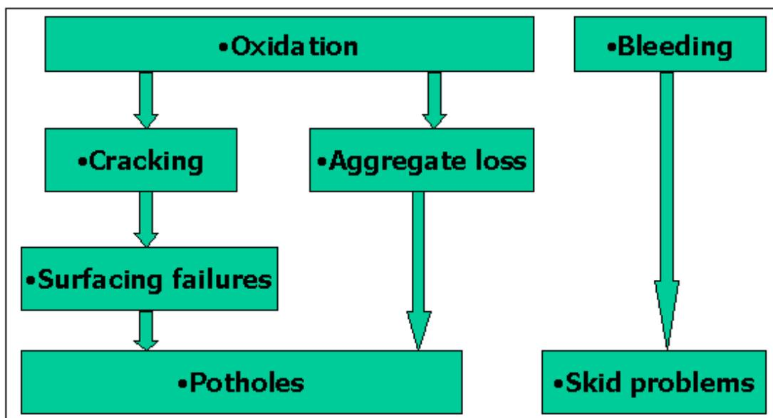
Figure 3. Surfacing deterioration.
