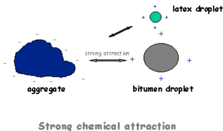
Figure 4. Chemical attraction of cationic SBR latex modified bitumen emulsion and aggregate.
