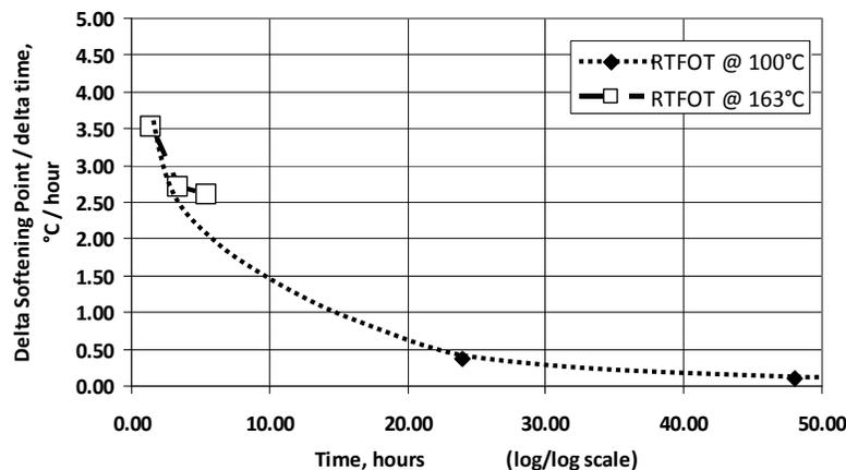
**Figure 5** Rate of ageing expressed by changes in Softening Point values (Extended RTFOT at 100°C and 163°C vs. PAV)
