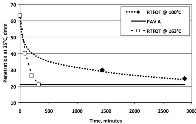
Figure 2 Relative Ageing measured by means of Penetration values (ERTFOT163 vs. ERTFOT100 vs. PAV)
