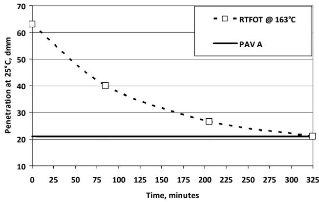
Figure 1 Relative Ageing measured by means of Penetration values
