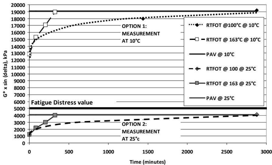
Figure 8 Accelerated Ageing measured with  $G^* \times \sin(\delta)$  at 10°C vs. 25°C (Comparing ERTFOT at 163°C, ERTFOT at 100°C vs. PAV)
