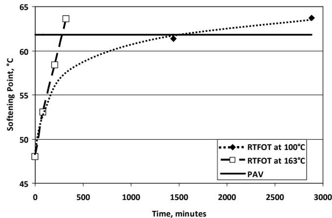
**Figure 4** Relative Ageing measured by means of Softening Point (Extended RTFOT at 100°C and 163°C vs. PAV)
