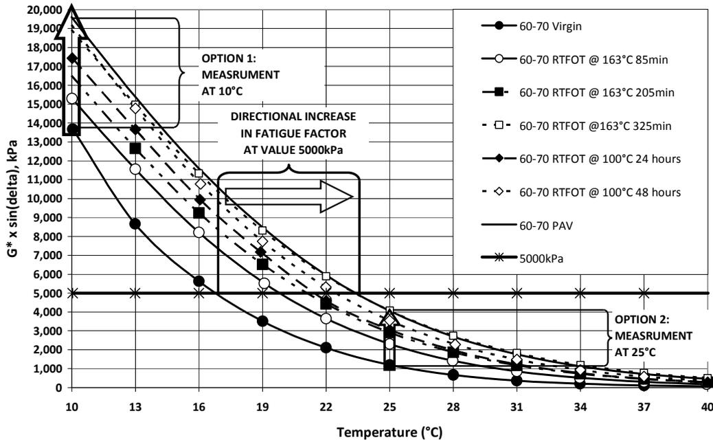
Figure 7 Comparison of the Complex Modulus ( $G^*$ ) between 10°C and 40°C
