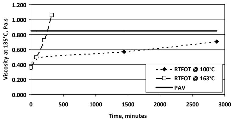
**Figure 6** Rate of ageing expressed by changes in Viscosity values at 135°C (Extended RTFOT at 100°C and 163°C vs. PAV)
