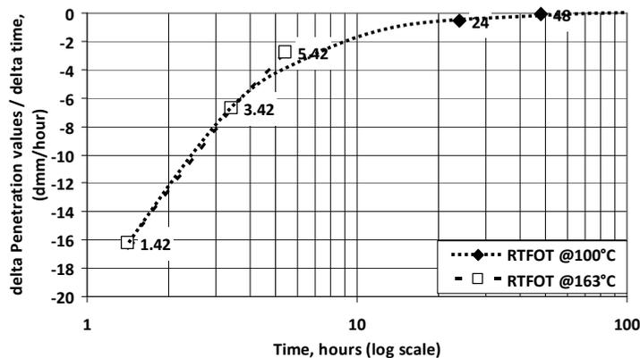
Figure 3 Rate of ageing expressed as changes in Penetration values at 25°C (Extended RTFOT at 100°C and 163°C vs. PAV)
