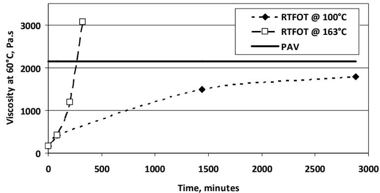
**Figure 5** Rate of ageing expressed by changes in Viscosity values at 60°C (Extended RTFOT at 100°C and 163°C vs. PAV)
