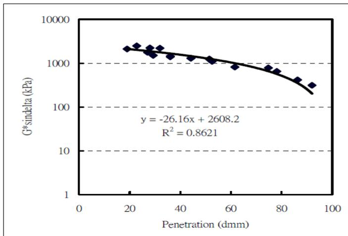
**Figure 3.** Relationship between Penetration values and  $G^* \sin \delta$  before and after the RTFOT and PAV at 25 °C (Lee *et al.*, 2004)
