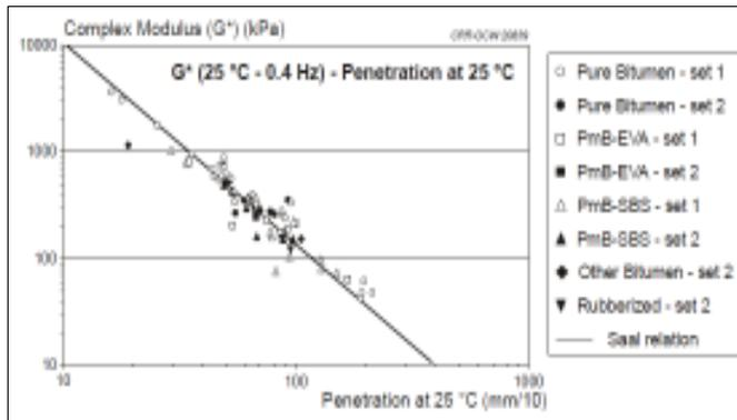
**Figure 1.** Binder modulus at 25 °C and 0.4 Hz versus Penetration values for about 100 binders of different origin (Gershkoff, 1995)
