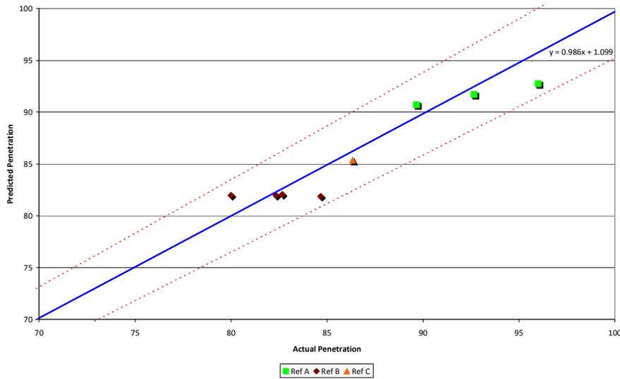
**Figure 7.** Actual Penetration versus Predicted Penetration using Model, plotted against Reproducibility Limits for ASTM D5
