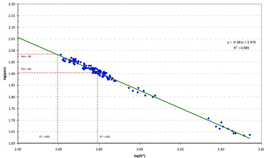
**Figure 4.** Relationship between  $\log(\text{Pen})$  and  $\log(G^*)$  at 25 °C penetration grade bitumen
