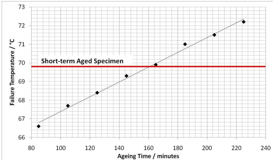
Figure 6: Failure temperature where  $|G^*|/\sin \delta = 2.20\text{kPa}$  against ageing time for the 40/50 binder.
