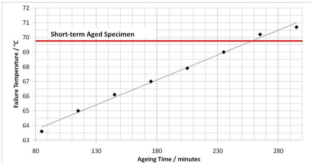
Figure 7: Failure temperature where  $|G^*|/\sin \delta = 2.20\text{kPa}$  against ageing time for the 60/70 binder.
