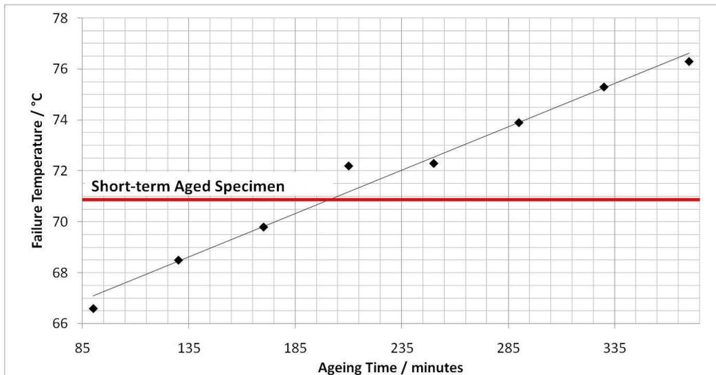
Figure 8: Failure temperature where  $|G^*|/\sin \delta = 2.20\text{kPa}$  against ageing time for the SBS-modified binder.
