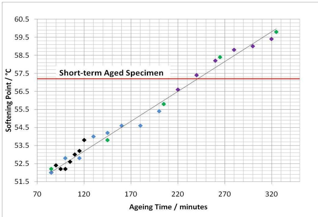
**Figure 4: Softening point data for aged 60/70 – separate colours represent four different data sets obtained on separate occasions**
