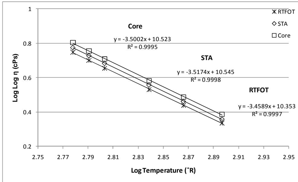
Figure 2: Viscosity-Temperature Relationships
