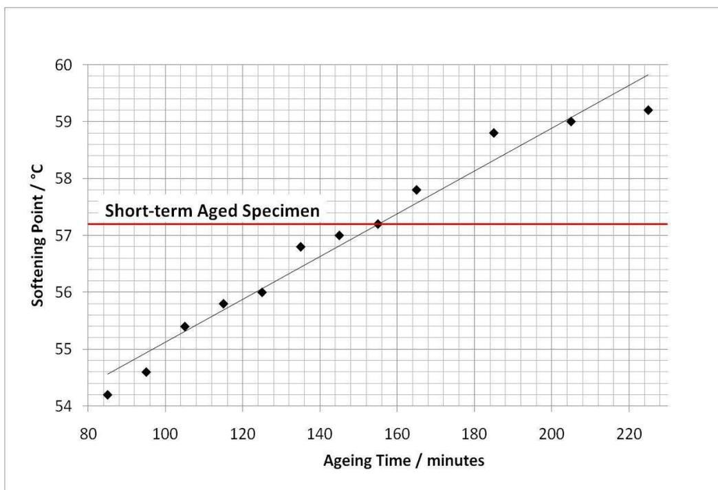
Figure 3: Softening point data for aged 40/50pen grade binder.
