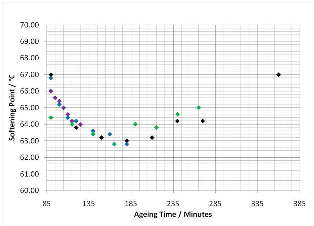
**Figure 5: Softening point data for aged SBS-modified binder – separate colours represent four different data sets obtained on separate occasions**
