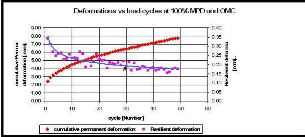
Figure 9. Development of the resilient and accumulative permanent deformation during a repeated load CBR test.
