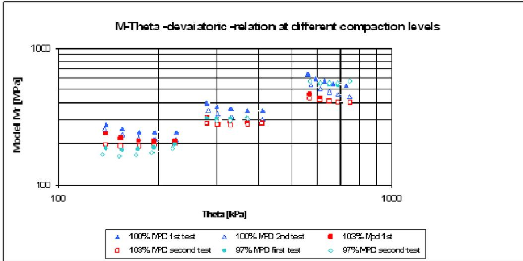
Figure 10. Stress dependency of the resilient modulus of the sand as determined by means of repeated load triaxial testing.
