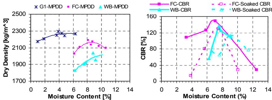
Figure 6. Moisture – density – CBR relationships for the tested granular base and subbase materials.
