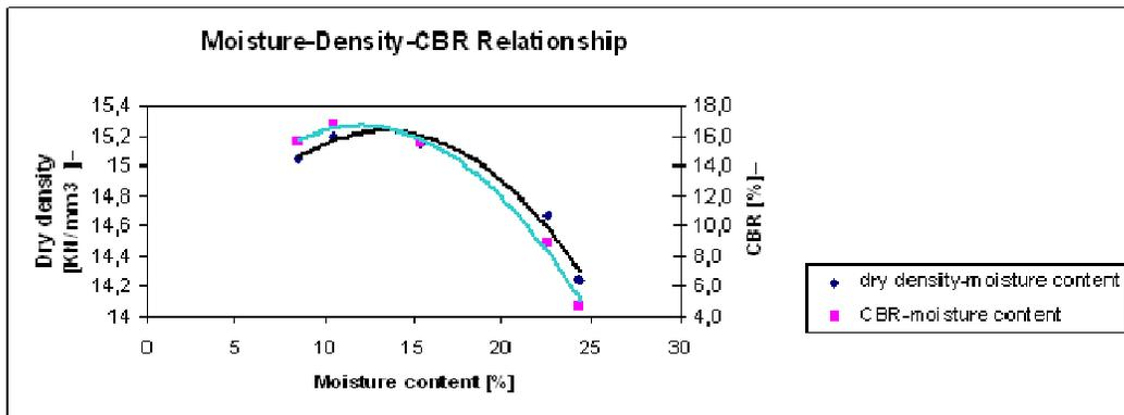
Figure 2: Moisture – density – CBR relationship for the tested sand.
