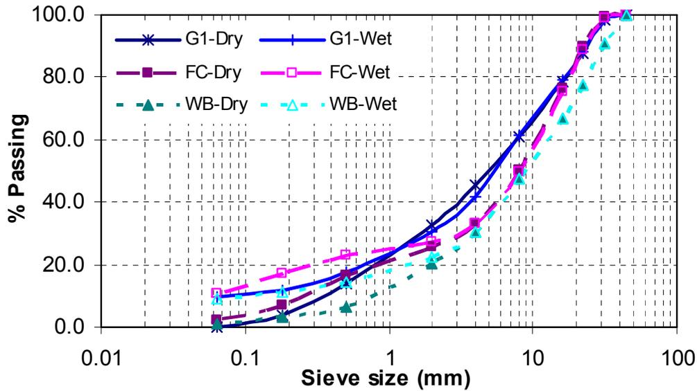
Figure 5. Gradation curves of the tested granular base and subbase materials.
