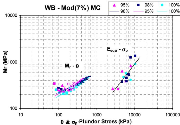
Figure 15. Comparison of resilient modulus vs. equivalent modulus typical example
