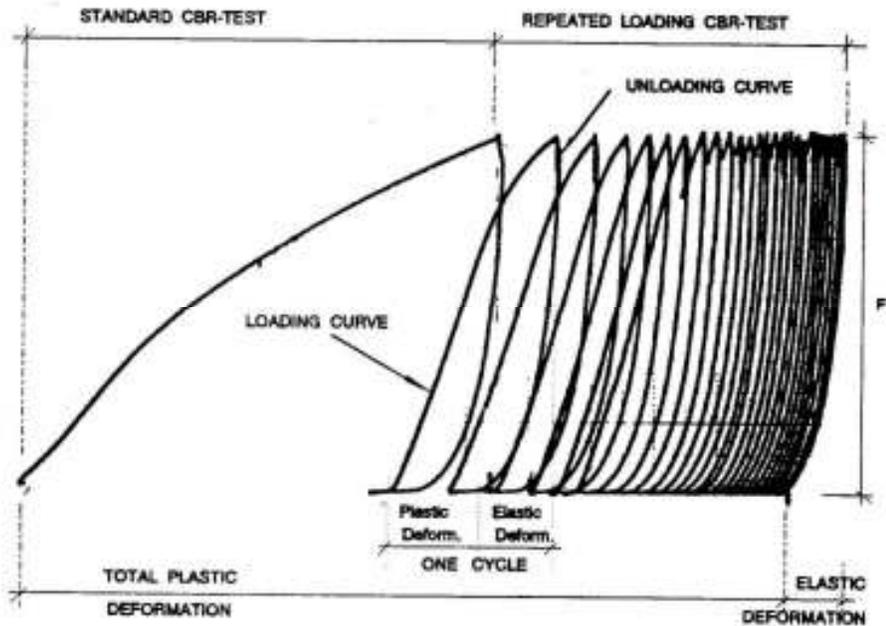
Figure 7. Example of the load – displacement curves obtained during a repeated load CBR test.
