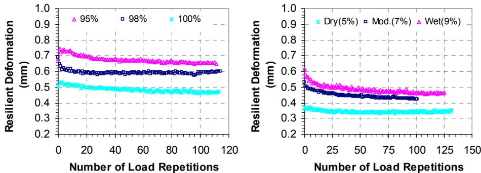
Figure 12. Effect of DOC at moderate MC and effect of MC at 95% DOC for WB.
