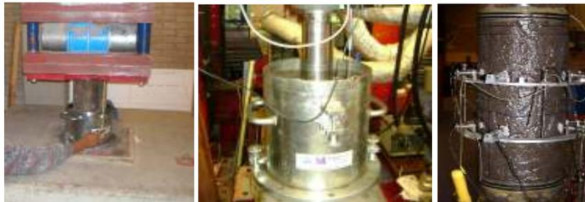
Figure 8. RL CBR specimen during compaction (left), RL CBR during testing (middle) and instrumented triaxial specimen ready for testing (right). All pictures relate to the coarse grained unbound aggregate specimens.
