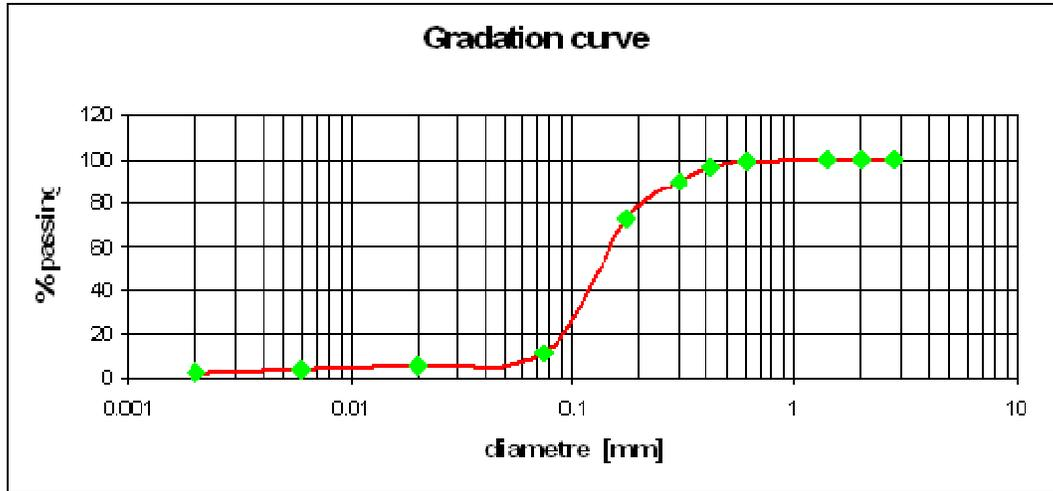
Figure 1. Gradation of the tested sand.
