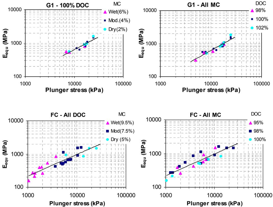
Figure 13. Stress dependent equivalent modulus for G1 and FC at various MC & DOC.
