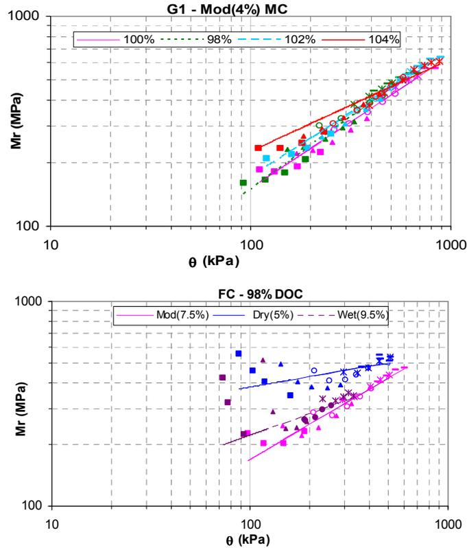
Figure 14. Examples of variation of  $M_r$  with bulk stress  $\theta$  DOC and MC.
