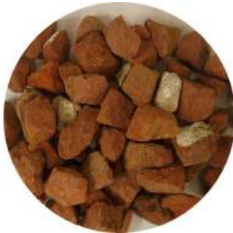
(a) Crushed masonry
