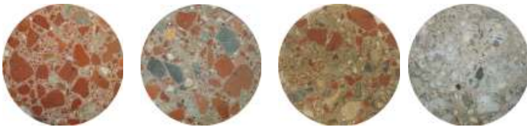
Figure 2. Cross Section of CTMiGr specimens (masonry content decreases from left to right).
