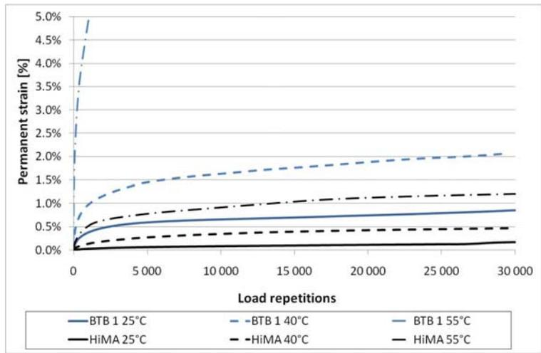
Figure 4: Permanent deformation HiMA compared to BTB
