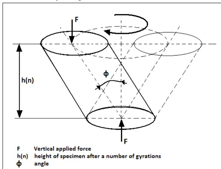
Figure 2: Configuration of a gyratory specimen during compaction
