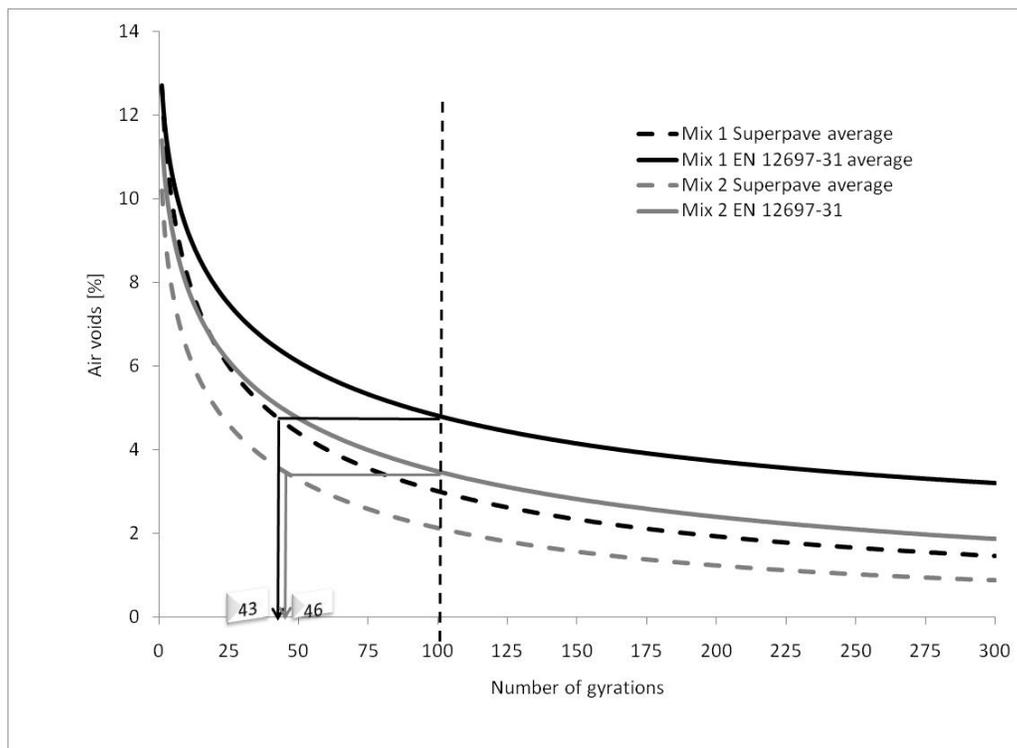
**Figure 3: Gyratory compaction curves for two mixes using European and SUPERPAVE configuration**
