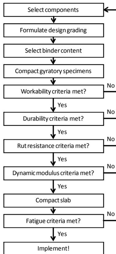
**Figure 1: Mix design process**
