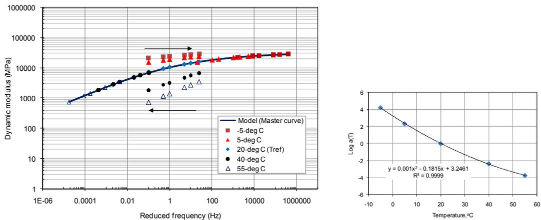
Figure 5a: Construction of a master curve for HiMA mix, b: Shift factors
