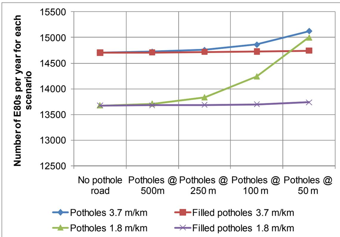
Figure 6: Comparison between actual E80s generated per year on IRI 1.8 m/km and IRI 3.7 m/km roads with filled potholes
