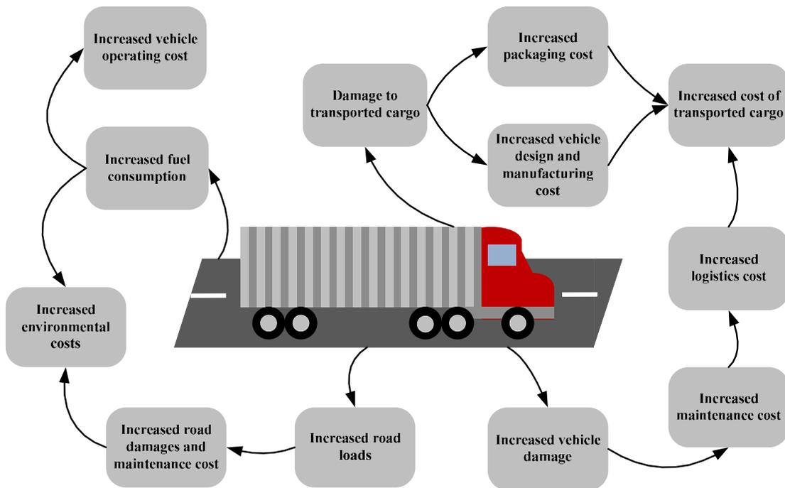
Figure 1: Conceptual indication of the effect of riding quality on truck logistics costs (Steyn et al, 2009)
