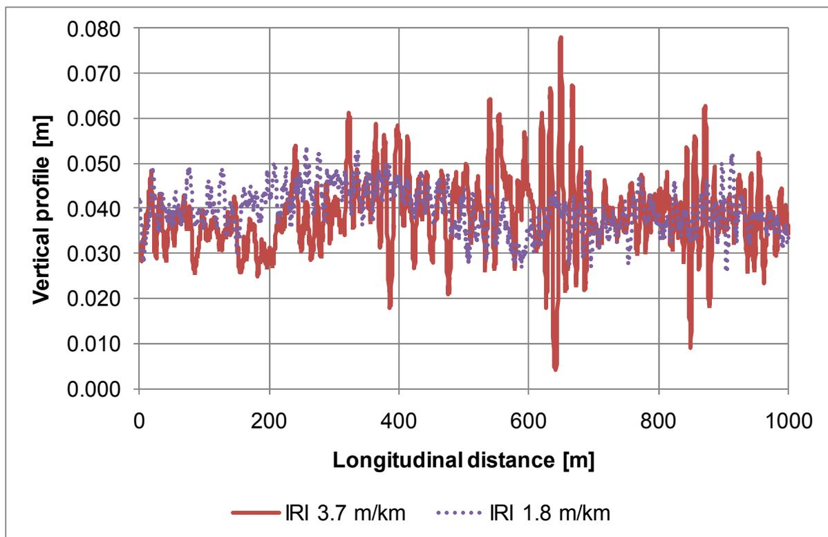
**Figure 3: Road profiles for two road sections used in the simulations**
