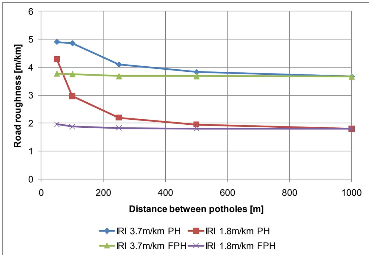
Figure 7: Effect of presence of potholes on road roughness (IRI)
