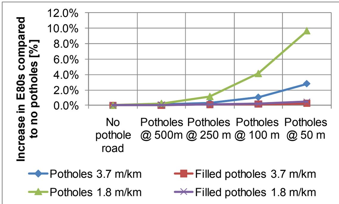
Figure 5: Percentage increase in E80s generated on IRI 1.8 m/km and IRI 3.7 m/km roads with open and filled potholes
