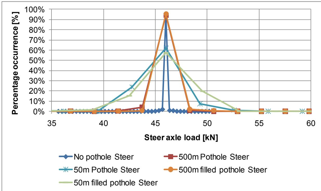
**Figure 4: Steer axle load distribution for IRI 1.8 m/km road section (only data between 35 kN and 60 kN shown for clarity)**
