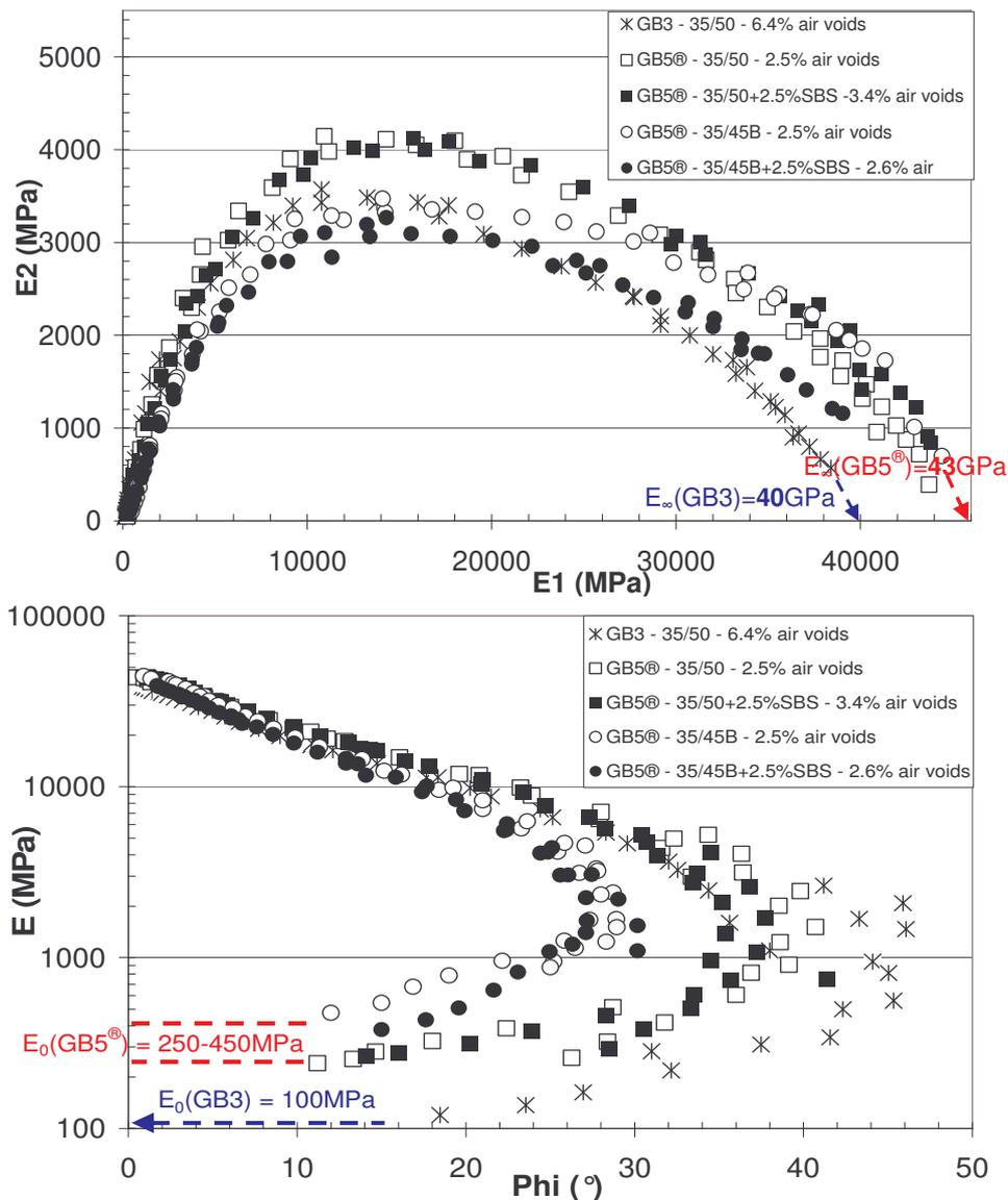
Figure 7 – Complex modulus results for GB3 & GB5 mixes (Cole-Cole and Black diagrams).
