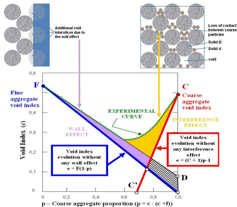
Figure 1 – Wall and interference effects, Powers [21].  $f$  and  $c$  are respectively the solid volumes of fine and coarse aggregates ( $f+c=1$ );  $F$  (resp.  $C$ ) = void index of fine (resp. coarse) aggregates.
