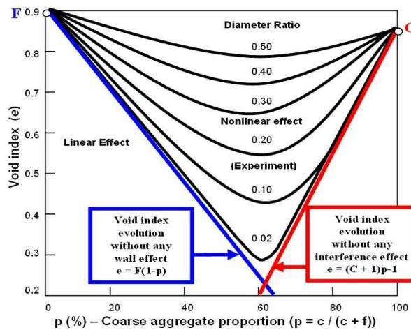
Figure 2 – Effect of diameter ratio ( $d_{FINE}/d_{COARSE}$ ) on void index ( $e$ ) of binary combinations of coarse ( $c$ ) and fine ( $f$ ) aggregates (Furnas [12], Powers [21], Oger [22] and Perraton [17]).
