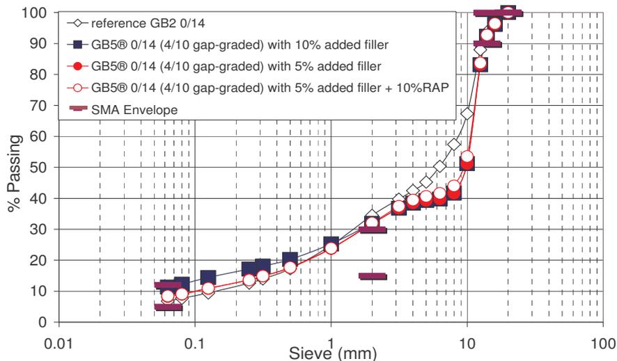
Figure 6 – Skip gradation curves (referred to as "GB5") for the optimal quaternary aggregate blends Vs that of the continuously graded reference "GB2".
