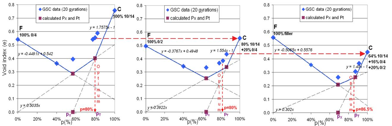
Figure 4 – 3-step iterative optimization of the 10/14-0/4-0/2-filler quaternary Nouveau aggregate blend.
