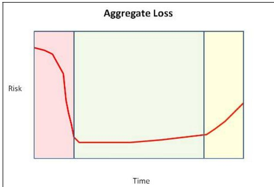
Figure 12 Risk of aggregate loss (Spray seals)
