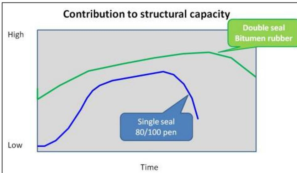
Figure 11 Seal contribution to pavement structural capacity
