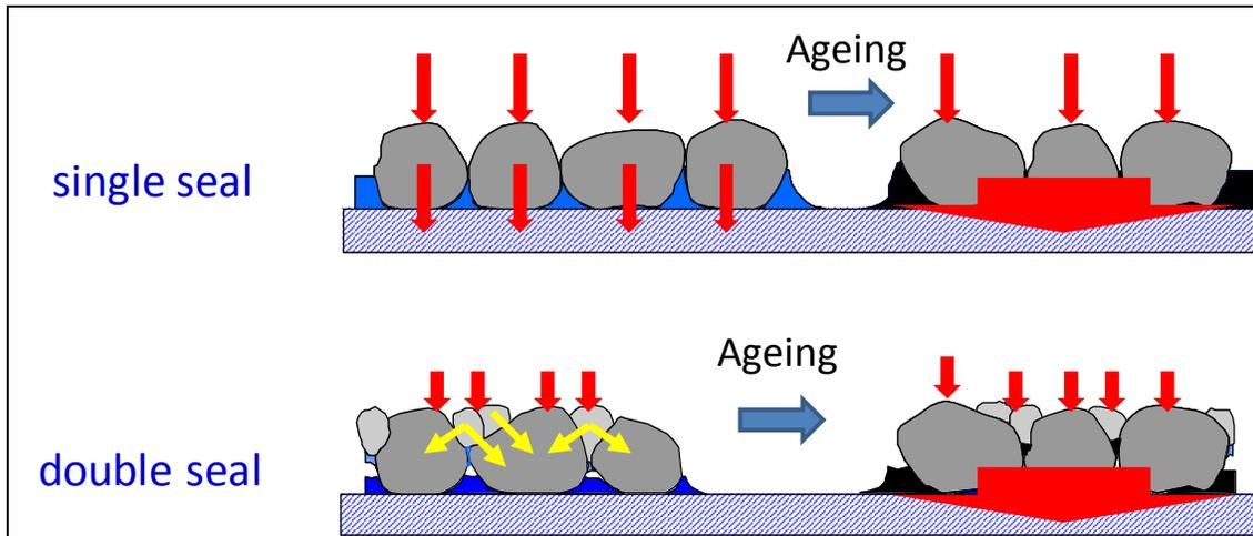
Figure 10 Effect of ageing on load distribution
