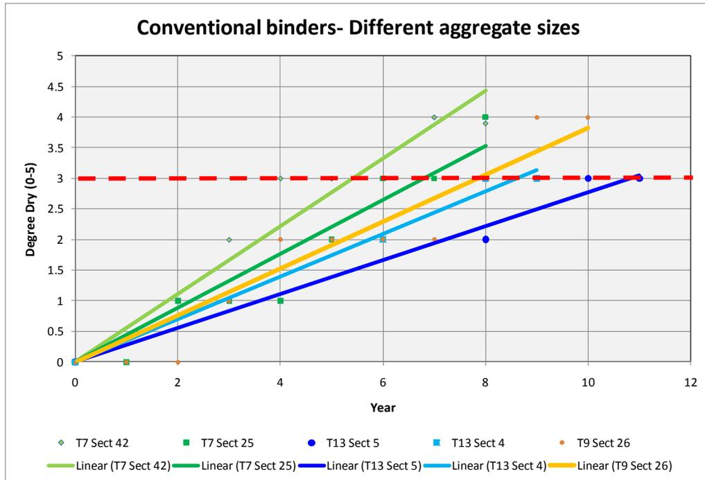
**Figure 3 Ageing as a function of aggregate size**
