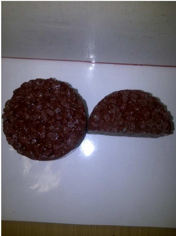
**Left:** UTFC with 5% red oxide, black binder and colour-coded aggregate
