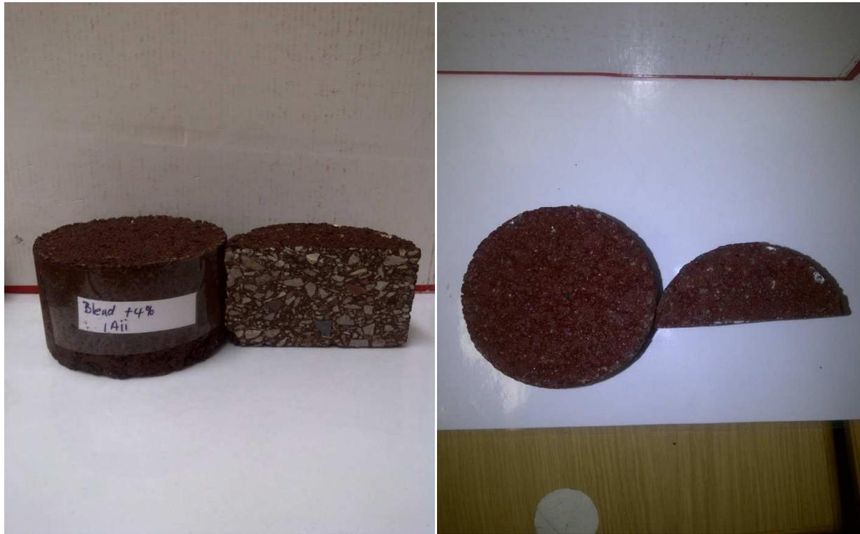
Figure 4: Option 2B(ii) from Table 1 (AC surfacing with red oxide colouring and 50% colour coded aggregate ex Durban)
