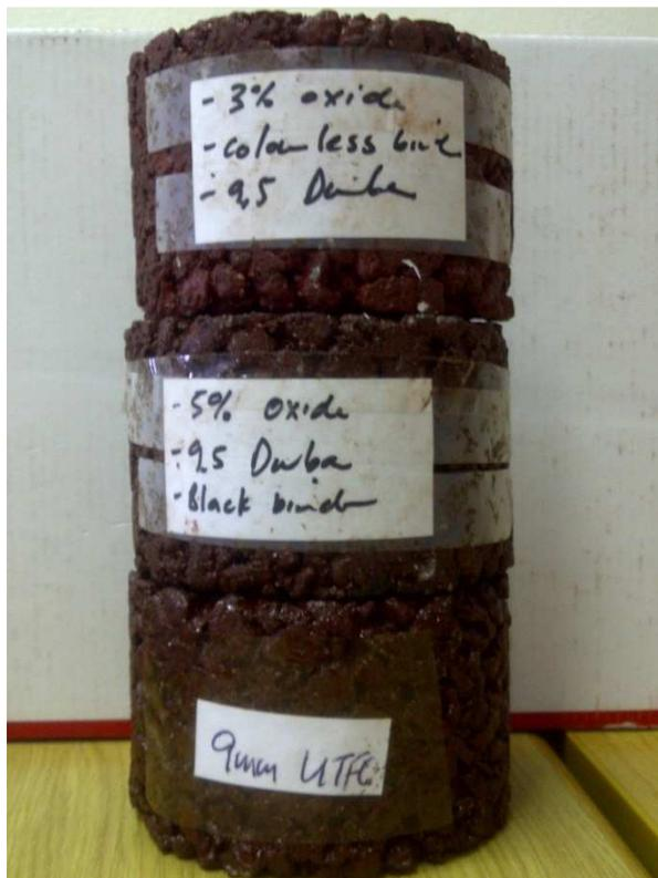
**Left:** Top briquette is UTFC with colourless binder, 3% oxide, and colour coded stone. Lower 2 briquettes are UTFC with Black Binder, 5% oxide and colour-coded stone.
