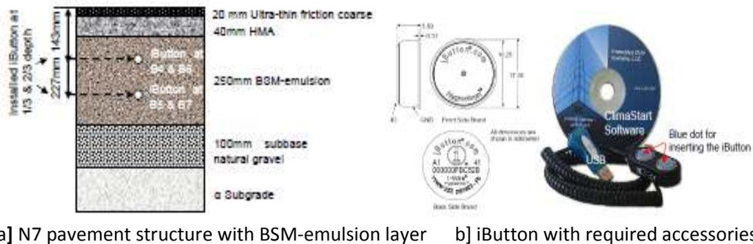
Figure 1: Pavement structure with BSM-layer, location of iButtons and accessories required for monitoring of temperature distribution
