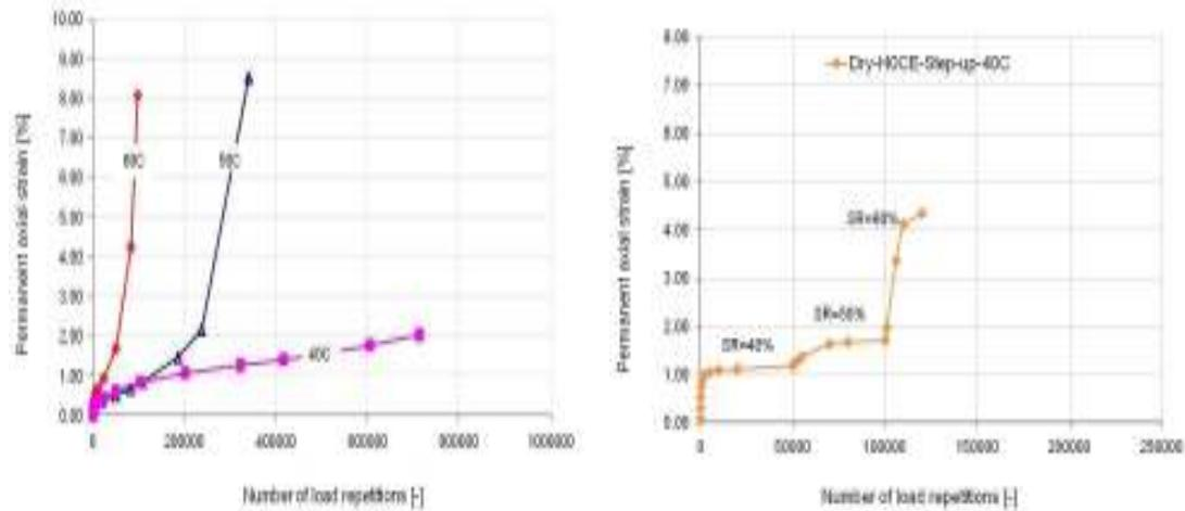
a) Permanent axial strain of field cores (BSM-foam) tested at SR of 40%, confinement 100kPa and active variable temperature. b) Multistage permanent axial strain on lab. spec (BSM-emulsion) with no filler and HOCCE tested at 40°C, confinement 100kPa and variable SR
