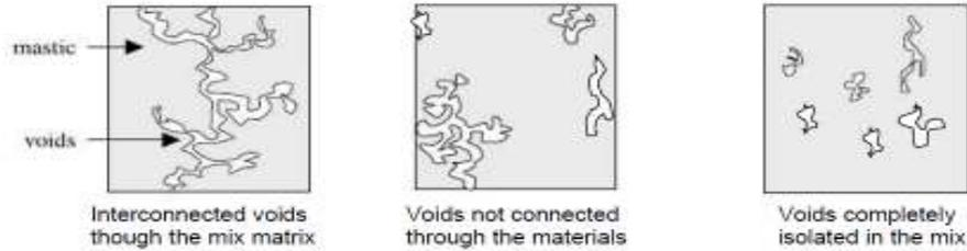
Figure 9: The different mode of voids structure present in the BSMs
