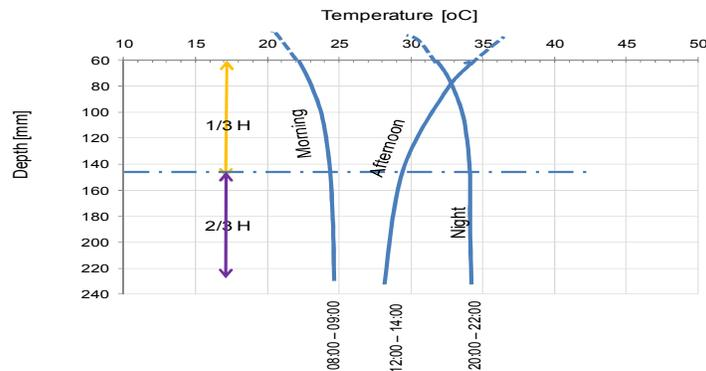
Figure 6: Temperature gradient through BSM-emulsion layer, with surface layer extrapolated
