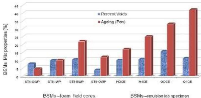
Figure 10: Comparison between air voids content and age hardening behavior in BSMs
