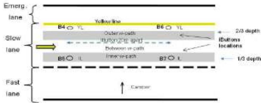
Figure 2: Layout and locations of installed iButtons in a BSM-emulsion layer at N7 expressway
