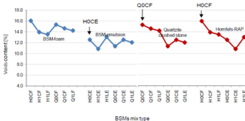
Figure 91: Voids properties of BSMs and influence of mineral aggregates types.
