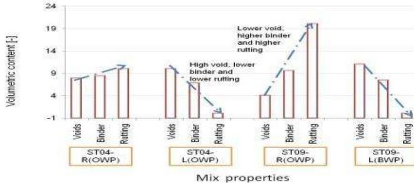
Figure 9: The relationship between voids content, binder content and rutting behaviour in BSM mixes from Shedgum Road
