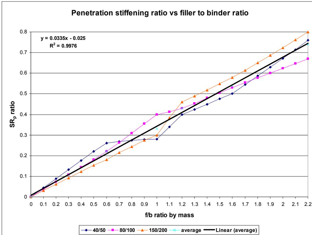
Figure 4: Penetration stiffening ratio versus filler/binder ratios (mass)
