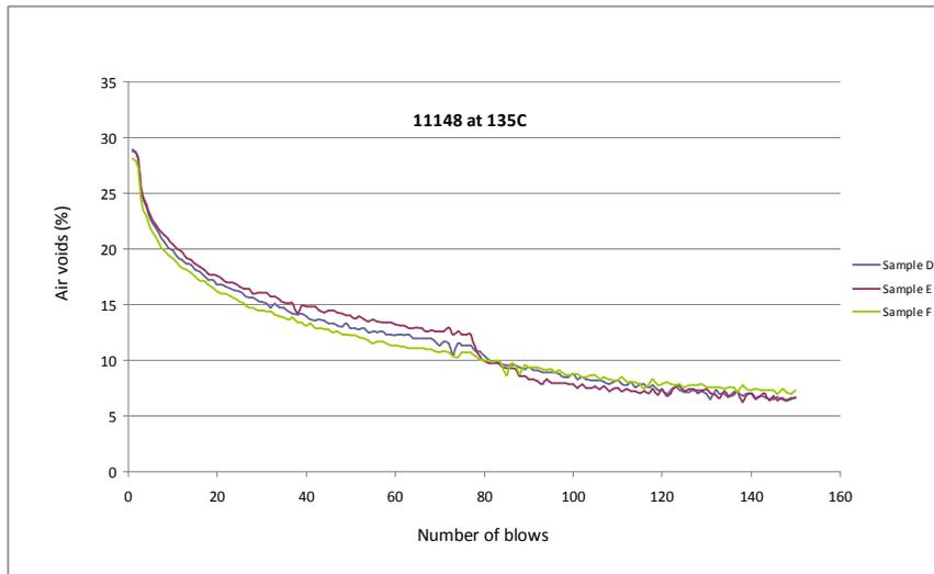
**Figure 2: Marshall compaction for material 11148 at 135°C.**
