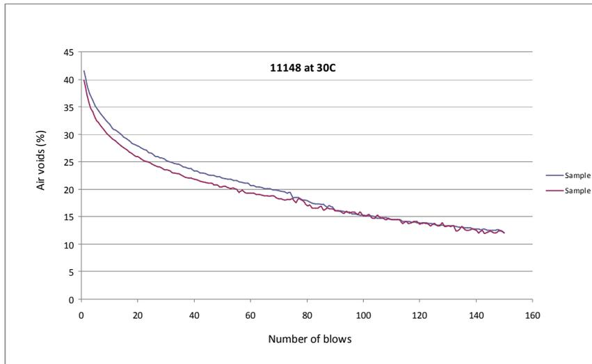
**Figure 1: Marshall compaction for material 11148 at 30°C.**
