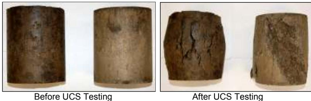
Figure 3/3A: FBS (3.0% bitumen % 1% Cement) V Cement-only (4<sup>+</sup>%) Briquettes
