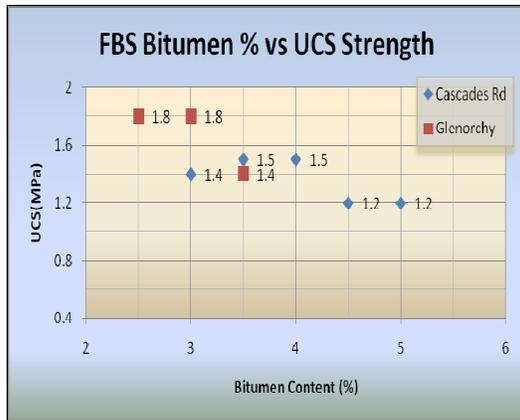
Figure 5: Bitumen % Vs UCS Strength
