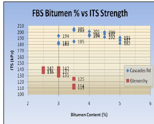
Figure 6: Bitumen % Vs ITS Strength
