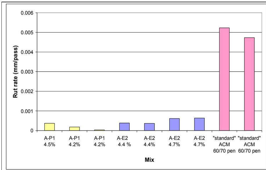
Figure 5: Comparison of Hamburg wheel tracking tests with other tested asphalt mixes.
