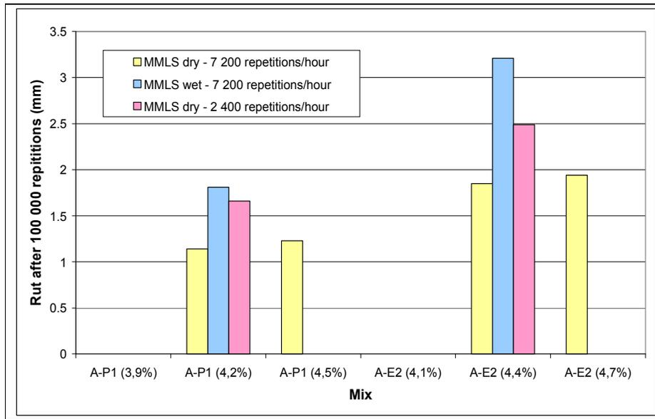
**Figure 3: Results from MMLS tests**
