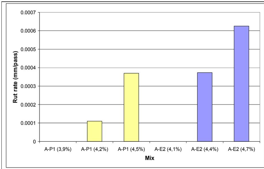
Figure 4: Result from Hamburg wheel tracking test
