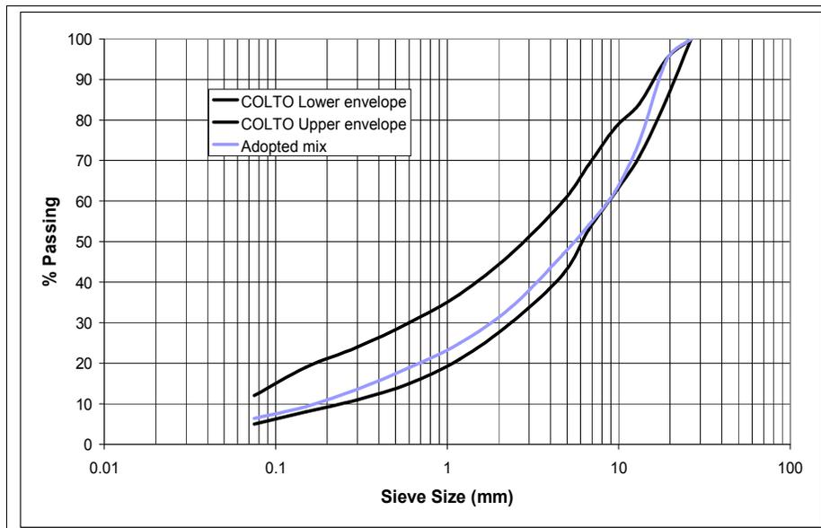
**Figure 2: Adopted mix grading vs. standard COLTO continuous grading**
