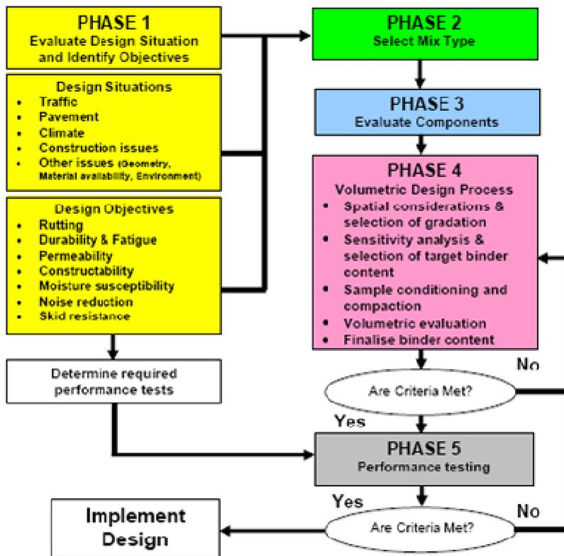
Figure 1: Standard Hot Mix Asphalt Design Process (HMA, 2001)
