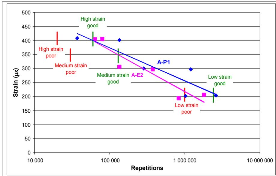
**Figure 6: Result from repeated bending beam fatigue tests**
