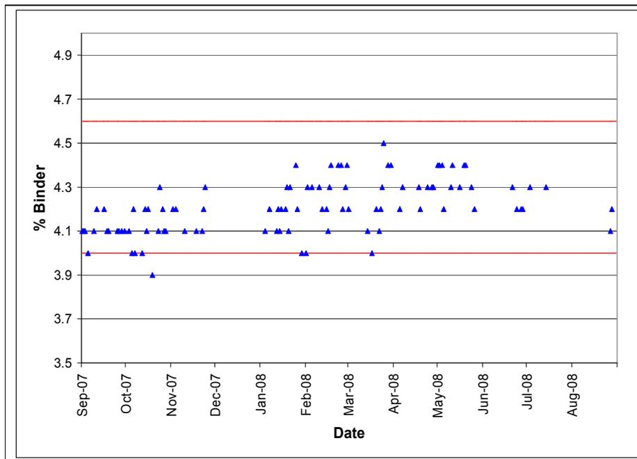
Figure 7: Typical daily Binder Content monitoring of production mixes during construction
