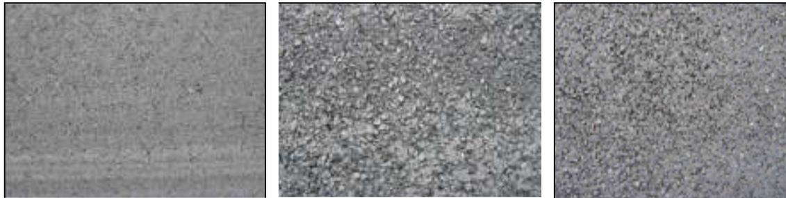
(a) Existing AC Surfacing                      (b) UTFC Layer (high Interconnected Voids)                      (c) BRASO (course and High Surface Voids)
