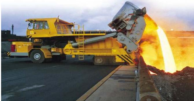
Fig2: Steel slag poured into a cooling bed
