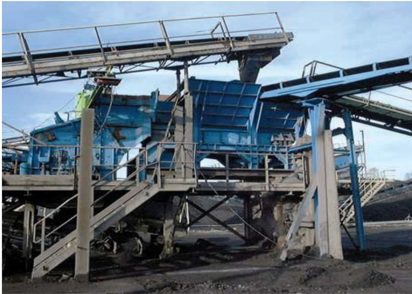
Fig.3: Grading machine for crushed steel slag
