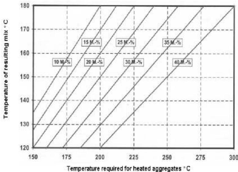
Fig.2: Required temperature for heated aggregates in °C for addition of dry RA at levels up to 10 and 40%M
