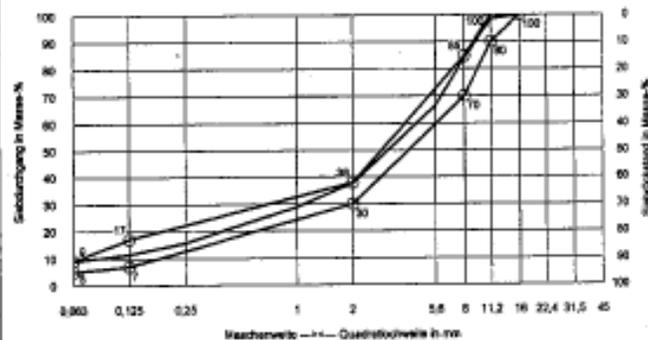
Fig.6: Grading curve for Polhornweg trial
