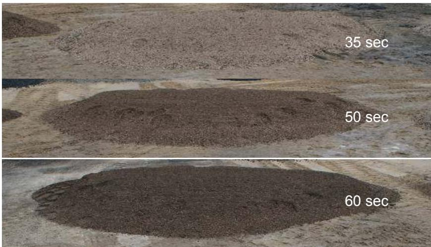
Fig. 1: 25% RA, mixed with superheated light coloured virgin aggregate
