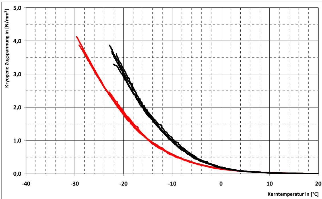
Fig.5: TSRT test data for binder layer mixes used in the Saseler Weg trial
