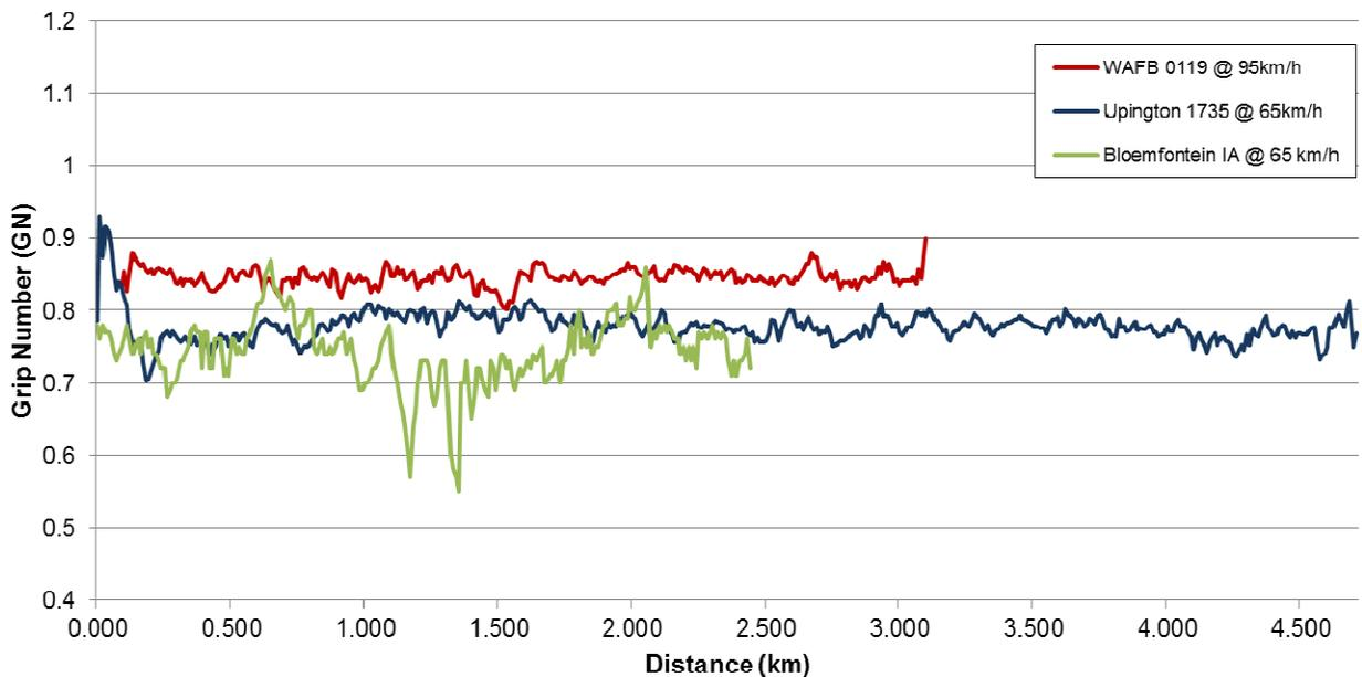
**Figure 11: Comparison of GN measurements of UTFC surfacing applied to South African runways**
