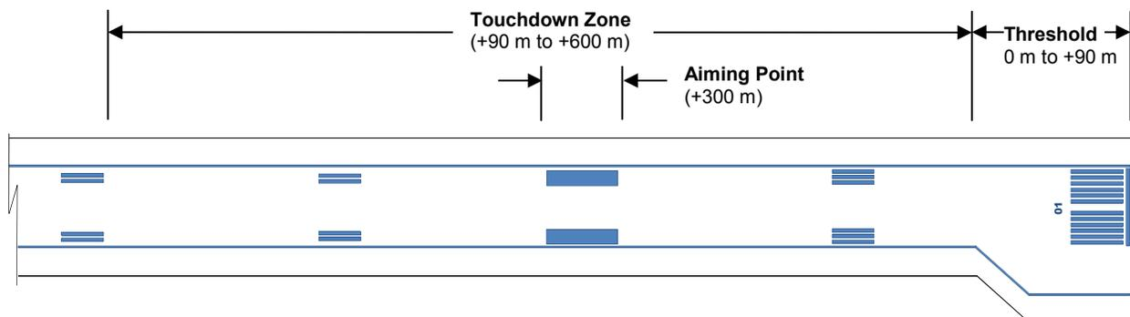
**Figure 2: Schematic representation of Threshold 01 of Runway 0119**
