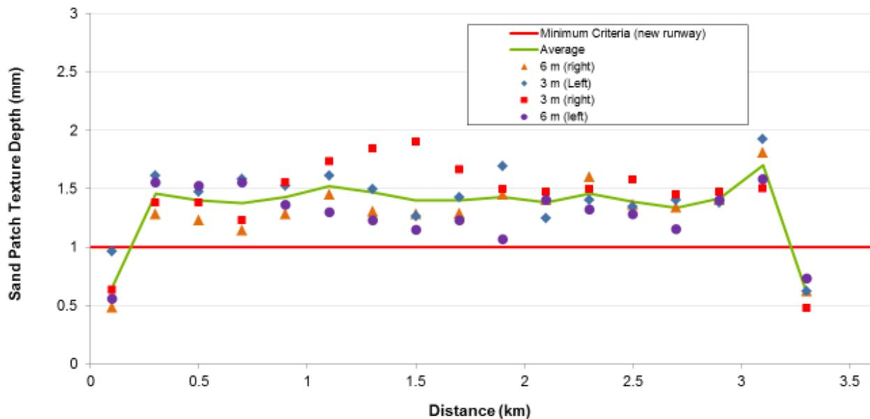
**Figure 9: Runway 0119 sand patch texture depth measurements**
