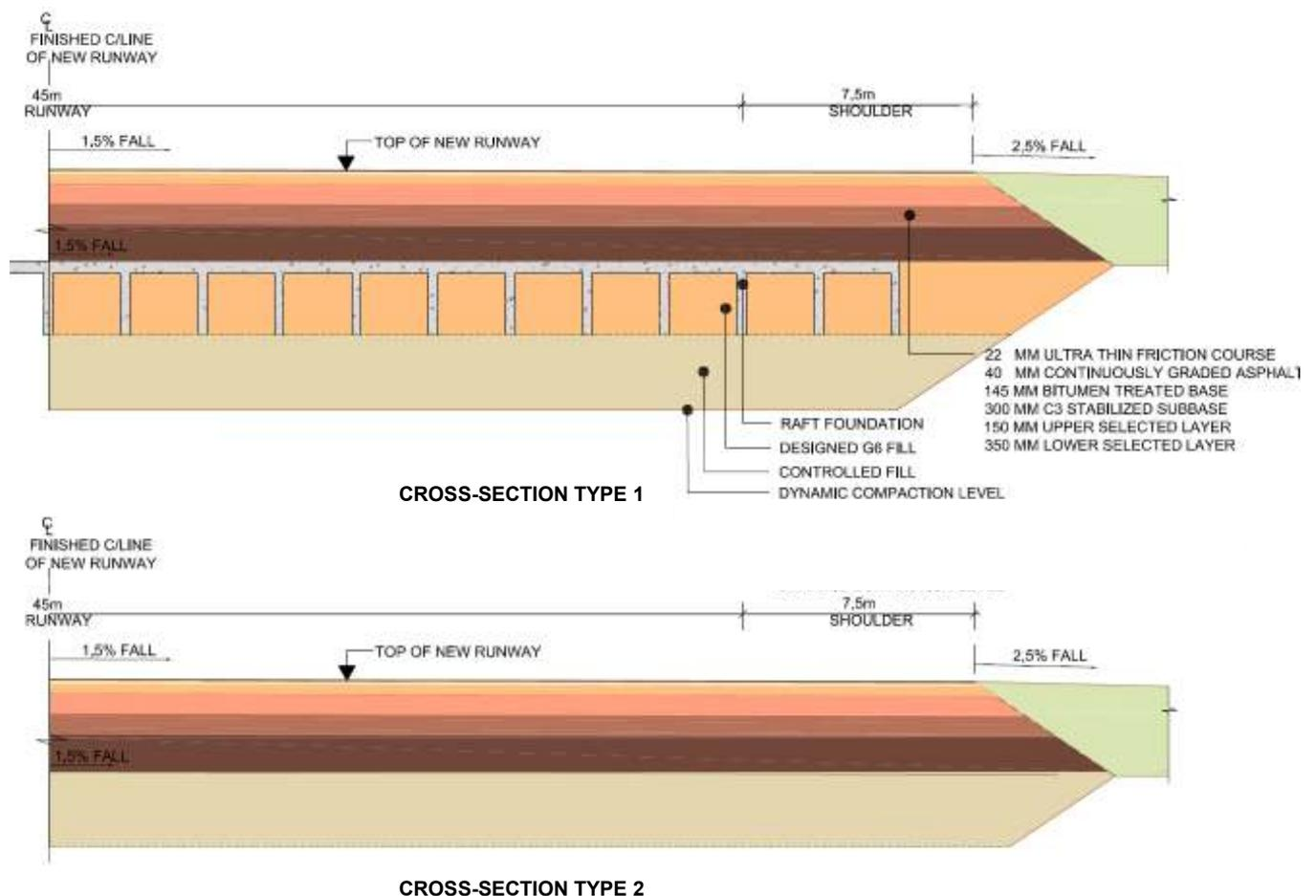
Figure 3: Substructure design incorporating raft foundation
