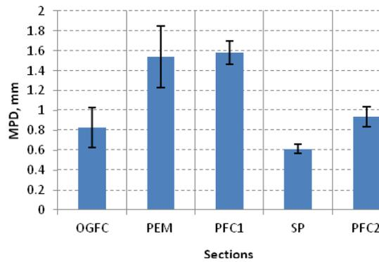
**Figure 4: Section Macrotexture Measurements**
