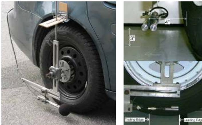
**Figure 1: The OBSI Method Microphone Configuration**
