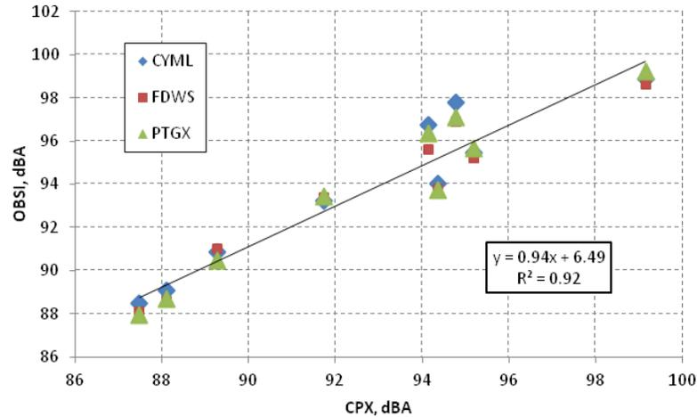
**Figure 7: Comparison of CPX and OBSI Sound Levels with the SRTT Tyre (45 mph)**
