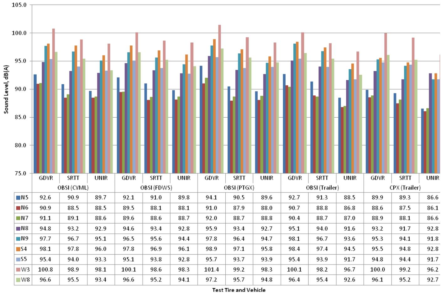
**Figure 6: Mean Sound Levels at a Speed of 45 mph**
