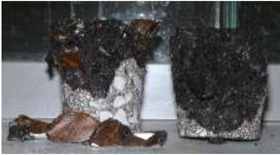
Figure 1. Compressive failure of the reference mixture (right) and the modified mixture with ceramic waste coarse aggregate (left).
