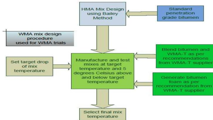
**Figure 4 Flow diagram for WMA laboratory mix design**
