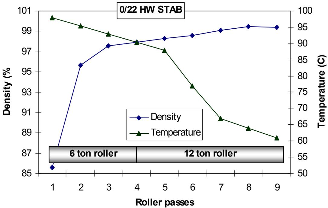
Figure 5. Compaction process for the LEAB base course mixture.
