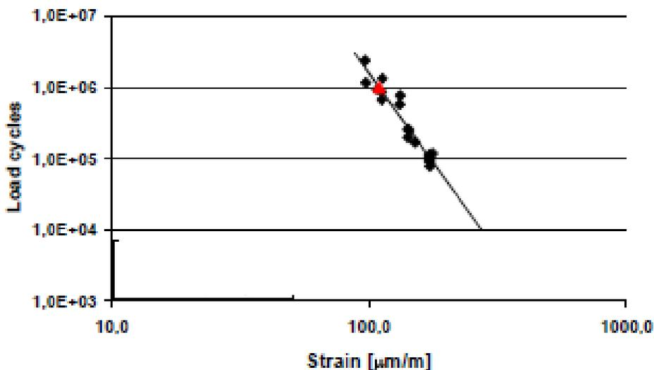
**Figure 3. Example of the fatigue tests on LEAB for CE marking (see regression line in table 3). The one million repetitions on the regression line is the required strain value  $\epsilon_6$ .**
