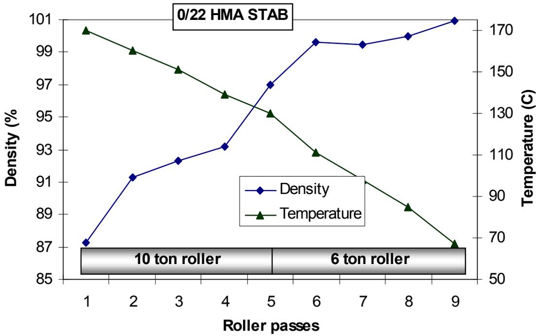
Figure 4. Compaction process for the hot base course mixture.
