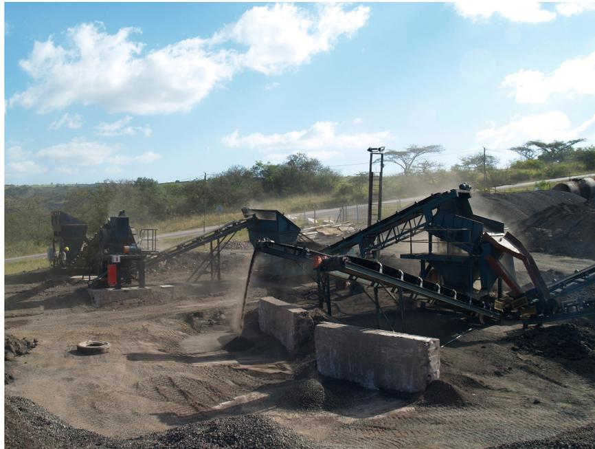
**Figure 4.1 Photographs showing preparation of the RA by crushing and screening**
