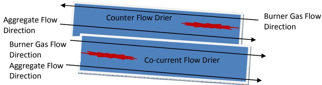
**Figure 2: Drier aggregate/burner gas flow direction arrangements**
