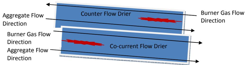
Figure 2 above indicates the two flow arrangements in terms of aggregate and burner gas in either a co-current (parallel) or counter-current arrangement.
